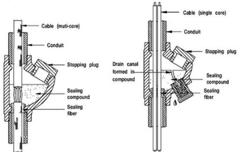
Fig 4. Encapsulation of Electrical Cable
