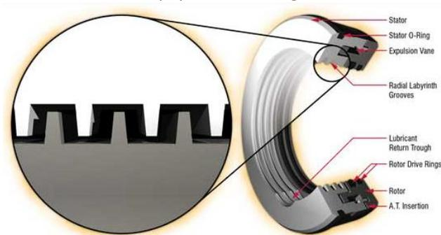
Fig. 3. Labyrinth seal of explosion proof rotating equipment
